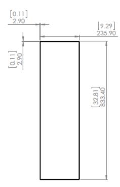
Cut Out Dimensions:7.6" W x 31.1" H Mounting Flange Width: 0.5" Finished Height above Drywall: 0.1" Bezel Width: 0.1"
